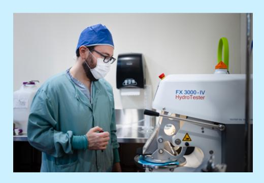
Testing water resistance: hydrostatic pressure
